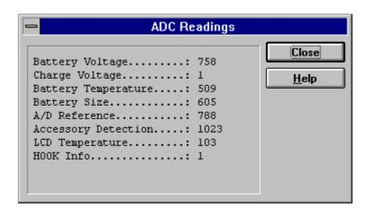
The **ADC Readings** dialog box has static text fields where measurements are updated to the window every one second.
